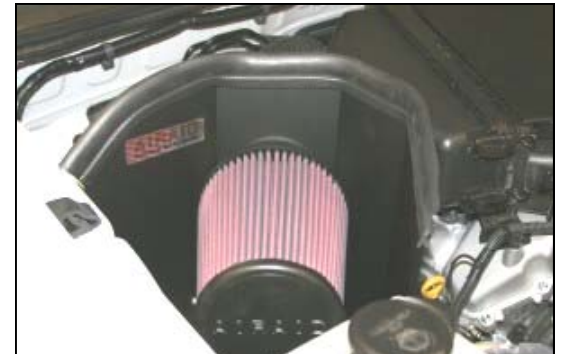
15. Install the Airaid Premium Filter (#1) on the CAD tube and tighten the clamp. Next install the weather strip (#7) on top of the CAD as shown. For an easier install, start at the fender side of the CAD and work your way towards the radiator.
